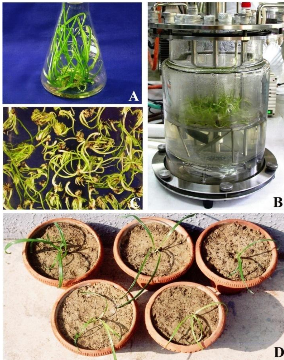
Figure 1. Propagation of C. borivillianum in bioreactor: in vitro regenerated shoots in liquid medium shake flasks from which explants were obtained (A), shoots cultured in bioreactor (B), shoot biomass harvested from bioreactor after 3 weeks of culture (C) and plants raised from bioreactor culture in earthen pots after 10 weeks of hardening (D).
